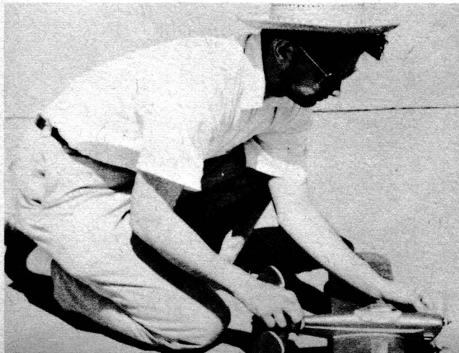
Though fuselage looks bulky for an .09, model has plenty of pep on a good engine. Larry listens to engine as he sets needle valve.
