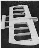
Turncoat basic structure shows "flex" section ribs for ease of building on a board, sheeted k.e. for strength and triple tailplane booms.
