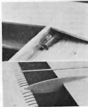
Wing tip detail shows outer tip, lead counter-balance weight buried in sheeting to prevent it coming out in a crash landing.
