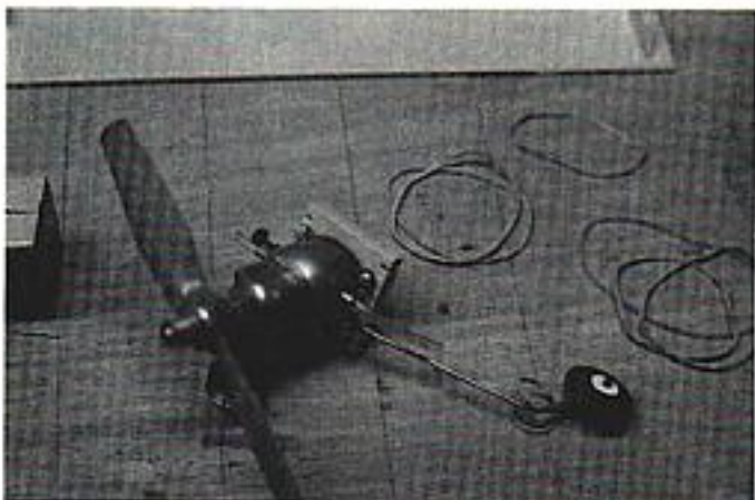
Left: The Cox .049 tank-mount engine screws to the plywood firewall with the nose gear wire sandwiched in between the two. The notches in the firewall are needed to give the rubberbands something extra to hold onto. Right: The bellcrank is mounted to a rather long plywood plate that also adds strength to the wing's center section. The main landing gear is clamped into place between the fuselage and the wing.
