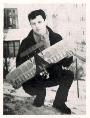
NORWEGIAN COMBAT RULES are now standardised as the F.A.I. 2.5 c.c. class regulations, and this model has been specifically designed and developed to suit the rules through several models to its final form as presented here. A.P.S. *Peacemaker* style swept back wing tips were found to give a definite improvement to its flying characteristics, mainly in the form of much smoother manoeuvres at high speed, the high speed being mainly due to the small wing area.
