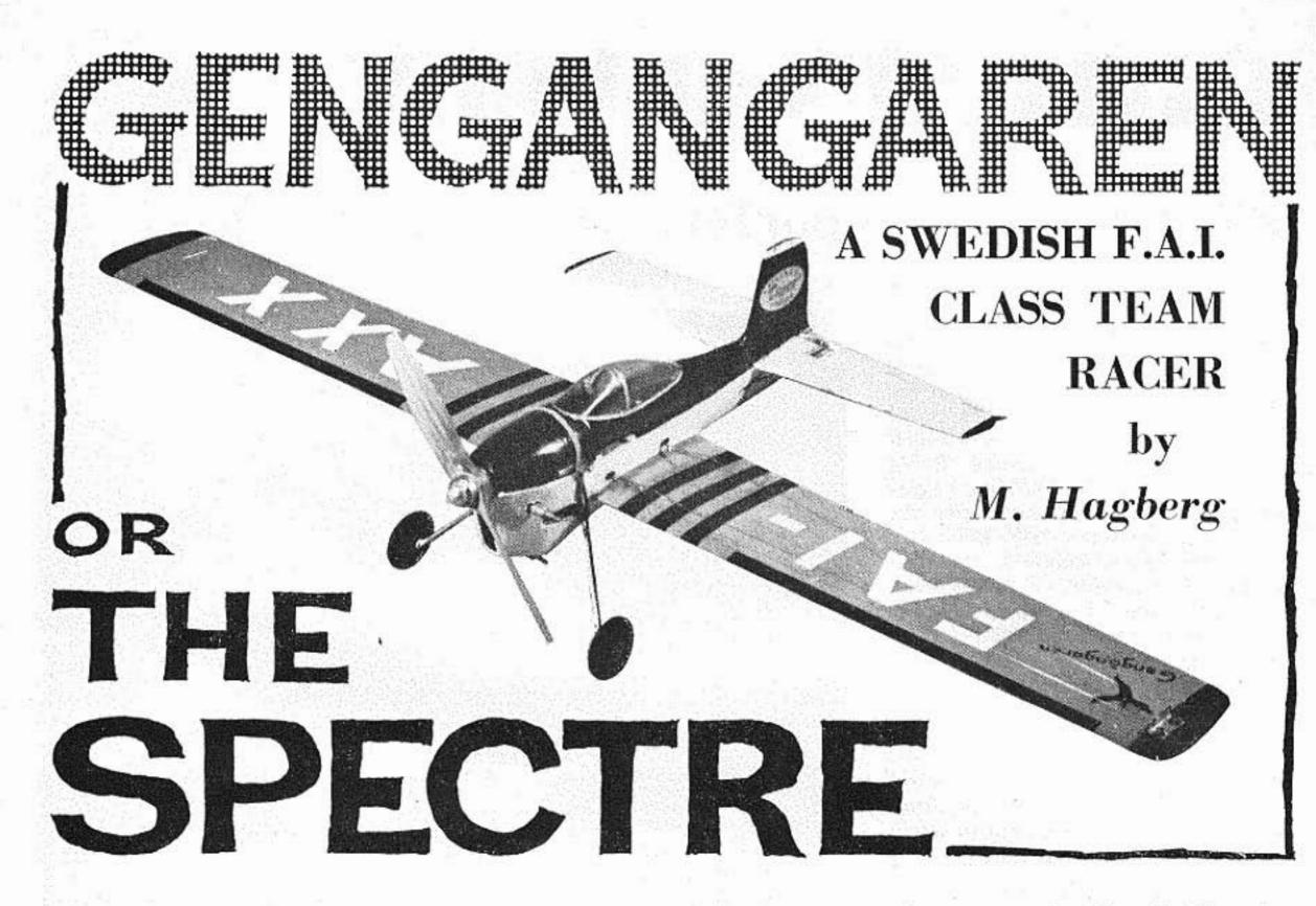
THIS model was designed with the following ideas in mind: 1. strength and reliability; 2. smallness, for low drag; 3. complete accessibility to tank and controls; 4. tank located to ensure positive starts; 5. control of oil seepage; 6. crankcase cooling, for consistent motor runs; 7. extremely quick and easy building; 8. good looks.
