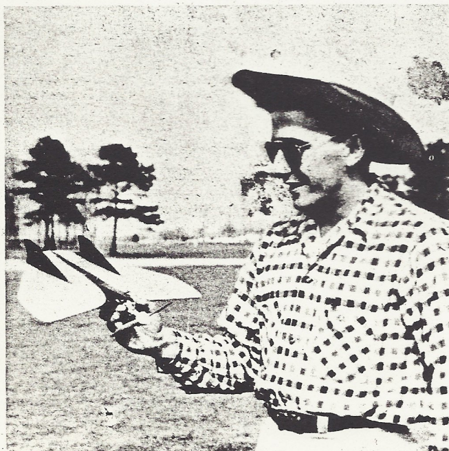
Perched on its master's hand, the docile bat shows twin tails. On 26-foot dacron lines, 6 x 3 prop, it's batty all right! You sharp?
