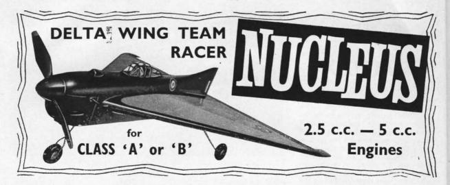
NUCLEUS is the development of four models, and though primarily designed for Class A racing, owing to its large wing area it can quite easily be converted into a Class B job by modification of engine mounting only. The Class A version with an E.D. Racer and 8 × 6 Stant prop has regularly clocked 75 m.p.h., while the Class B version with an O.K. Hothead, has been timed at 95 m.p.h. The model is very stable and easy to fly, and it is an ideal trainer for the newcomer to C/L flying.
